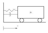
$$m\ddot{x} = -\underbrace{b\dot{x}|\dot{x}|}_{\text{damping}} -\underbrace{k_0x - k_1x^3}_{\text{spring}}, \qquad b, k_0, k_1 > 0$$
