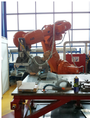
Figure: FSW at TWI in Sheffield
