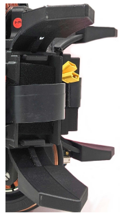
6. Four lipo battery slots, each 12.6 volts
