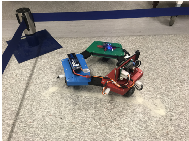
(a) Robot frame, raspberry pi, battery, servos, crazyflie
